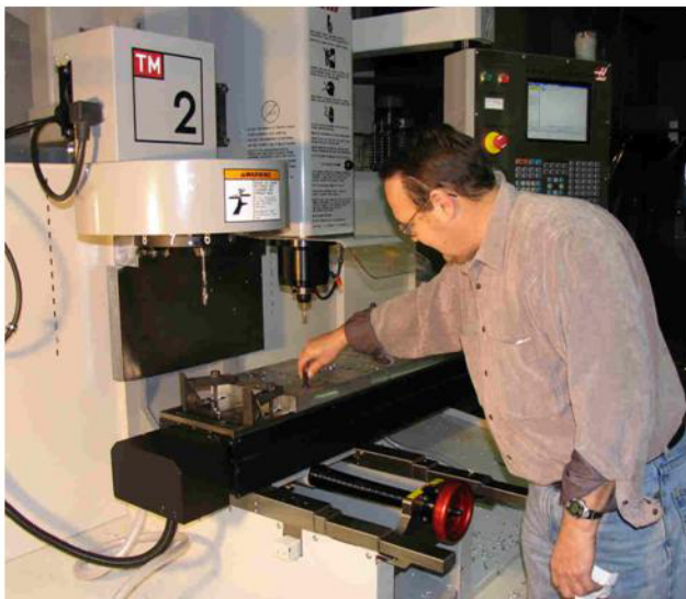
Left: Cliff Metger, Director of Engineering, checks out the Haas TM-2. Right: Close look at a milling job in progress. This particular piece of work saved the company about $500 in shop fees and two weeks in turnaround time.
